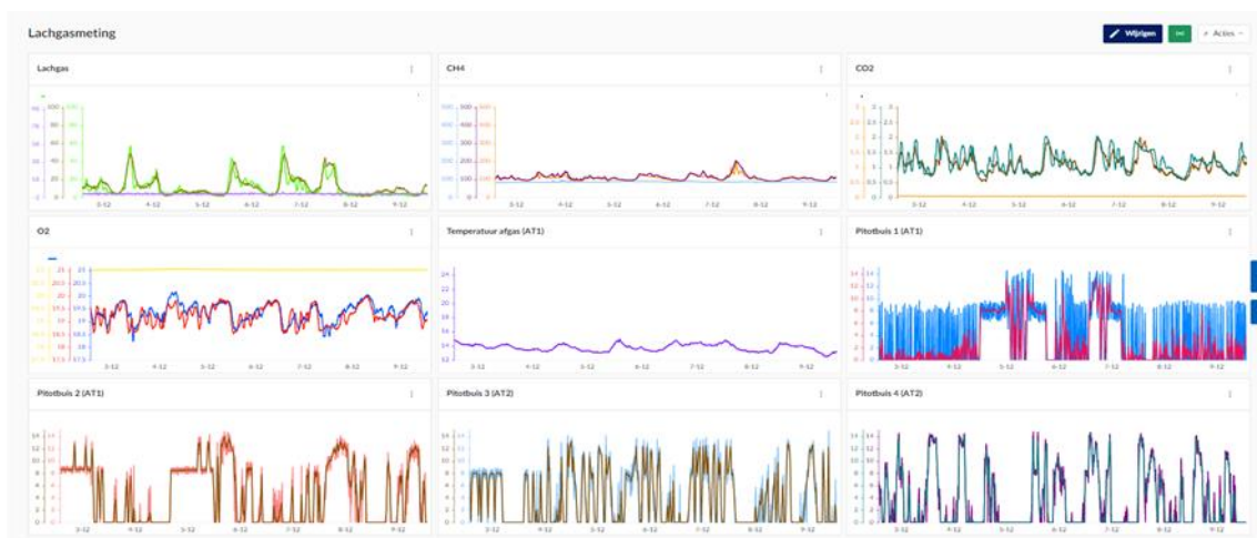
Fig. 3 Dashboard example with off-gas measurements (Nitrous oxide, methane, carbon dioxide and oxygen) and parameters relevant for off-gas measurement.
